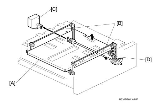
This tray mechanism is basically same as the tandem LCT. This tray bottom plate [A] is lifted through the tray wires [B] by the lift motor [C] rotation. There is no remaining paper capacity detection.
